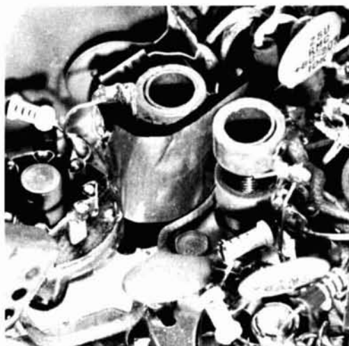
fig. 4. The decoupling tab between coils L3 and L4 increases circuit Q.
